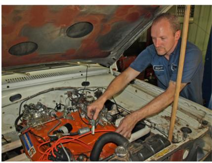
September in Massachusetts. Ambient temperature of nearly 100-degrees, plus nearly unbearable humidity limited our testing. With the distributor set to deliver 35-degrees BTDC at 3,000 rpm, the Orange box delivered 343.24 hp and 370.79 lb/ft to the tires. All runs were made with the Torqueflite in Drive and Bunky flooring the gas pedal at 3000 rpm and holding it there until the test concluded at 6,000 rpm.
