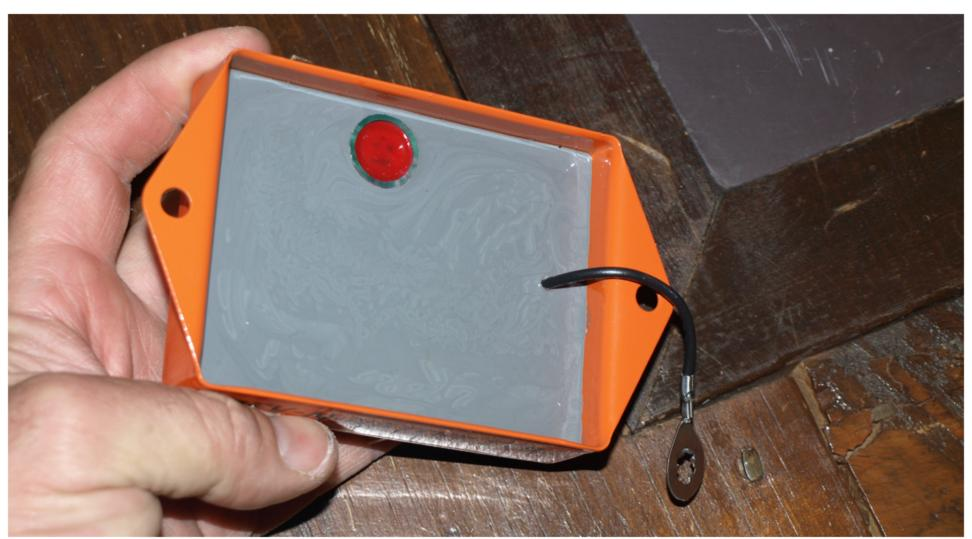
The backside is potted with a pliable rubber-like material to protect the electronics from moisture and vibration. The ground wire is unique to the Rev-N-Nator. The R/T Garage says the electronics are superior to factory items and that 10 to 40 extra horsepower are typically unleashed – after ignition timing is retarded a few degrees to accommodate the characteristics of the Rev-N-Nator.
