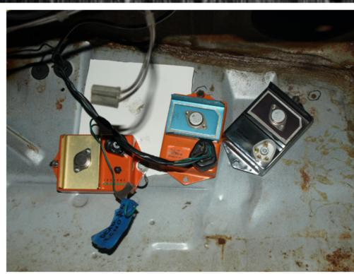
This close up shows how I temporarily mounted all three ECU's close together so we could jump between them quickly during the test. The contenders are (L to R) the Rev-N-Nator (PN OR #526), MP Orange box (P4120505) and MP Chrome box (P4120534). The Rev-N-Nator is the only unit requiring an external ground wire. Note the correct ground wire orientation with the lead pinched between the mounting ear and bolt head.
