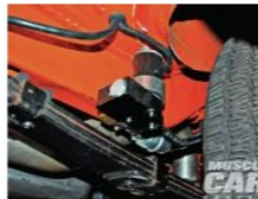
To push much-needed octane up to the mechanical pump from the tank, Al installed an Edelbr
