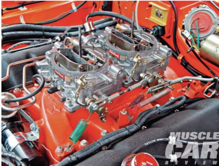
The two Edelbrock 600s work in unison to get the big Hemi the octane nourishment it needs. They are stacked single file on the original-issue intake. Check out the linkage—complex to the eye, but well thought out and executed.
