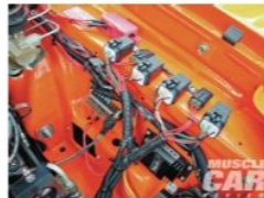
The Painless wiring system might be an eyesore to purists, but it does the job, “harnessin
