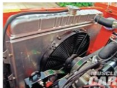
Al's dual Spal fan setup is digitally controlled. The interior engine bay puller fan comes
